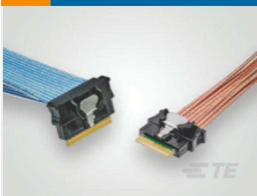
TE 产品编号 2820397-1 SLIVER C/A, 50P, STR TO STR, 10GHZ, 85OHM
