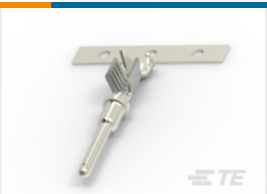
TE 产品编号2098252-3 PIN, SF, SIZE 16, 14-16 AWG, NI/SN
