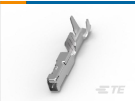
TE 产品编号2098762-4 Contact,female0.64, 22 AWG, CuNiSi, Sn
