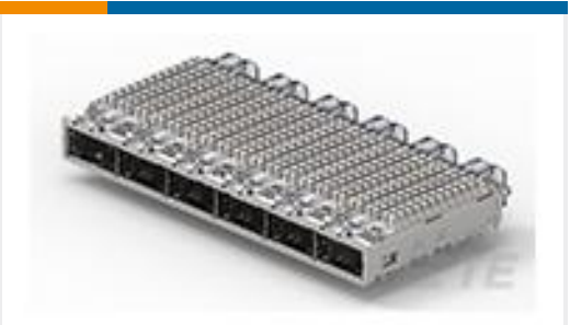
TE 产品编号 2143331-5 1X6 CAGE ASSEMBLY, BEHIND BEZEL, W/ SQR
