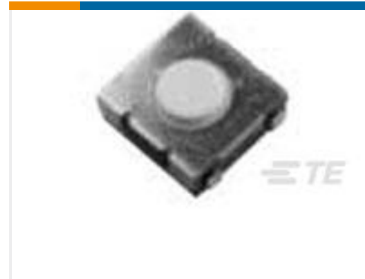
TE 产品编号 1571625-2 TACT,6X6,SMT,J-LEAD,50GF,T&R
