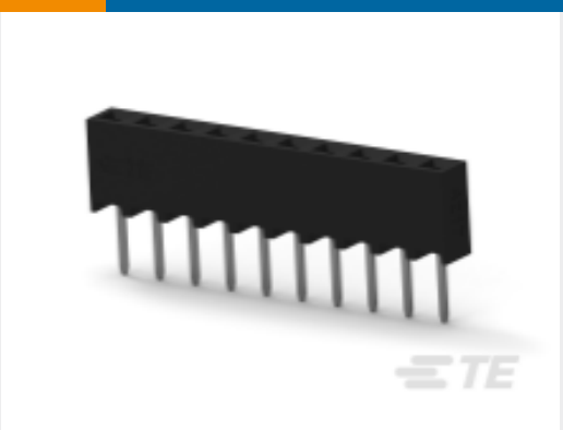
TE 产品编号1-2314868-0 10P,2MM,BB,REC,SRVT,2.0,0.1AU,TB,W/CP
