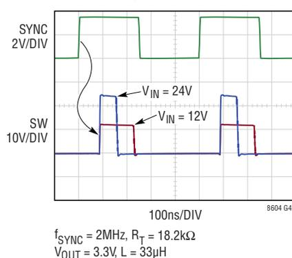
**LT8604C: Transition between Burst Mode and Forced Continuous Mode**
