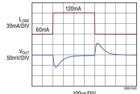
12V<sub>IN</sub> TO 5V<sub>OUT</sub>, LT8604C, SYNC FLOATING
