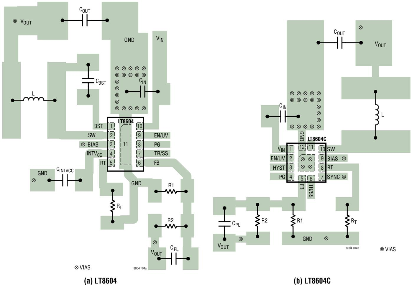
Figure 4. Recommended PCB Layout (Not to Scale)
