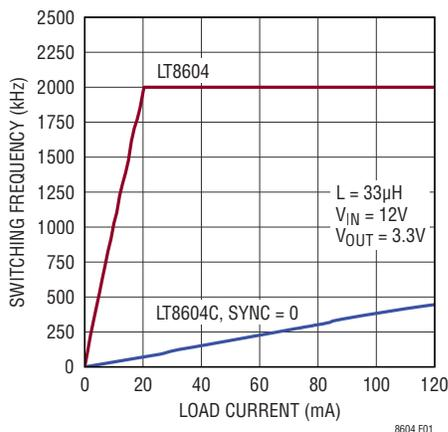
Figure 1. SW Burst Mode Frequency vs Load
