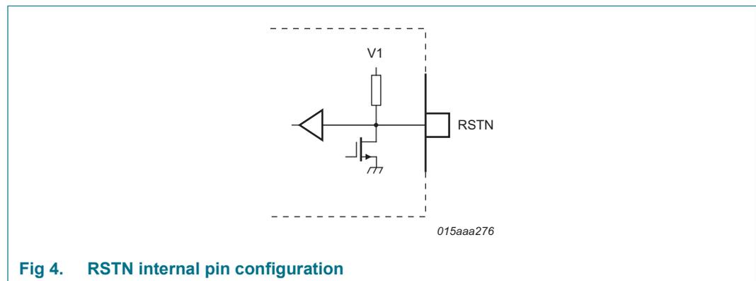
Fig 4. RSTN internal pin configuration
