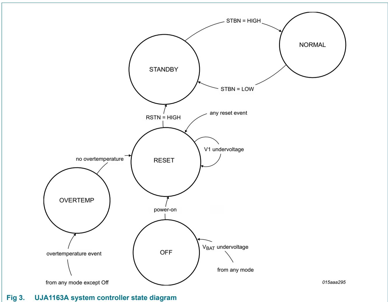
Fig 3. UJA1163A system controller state diagram
