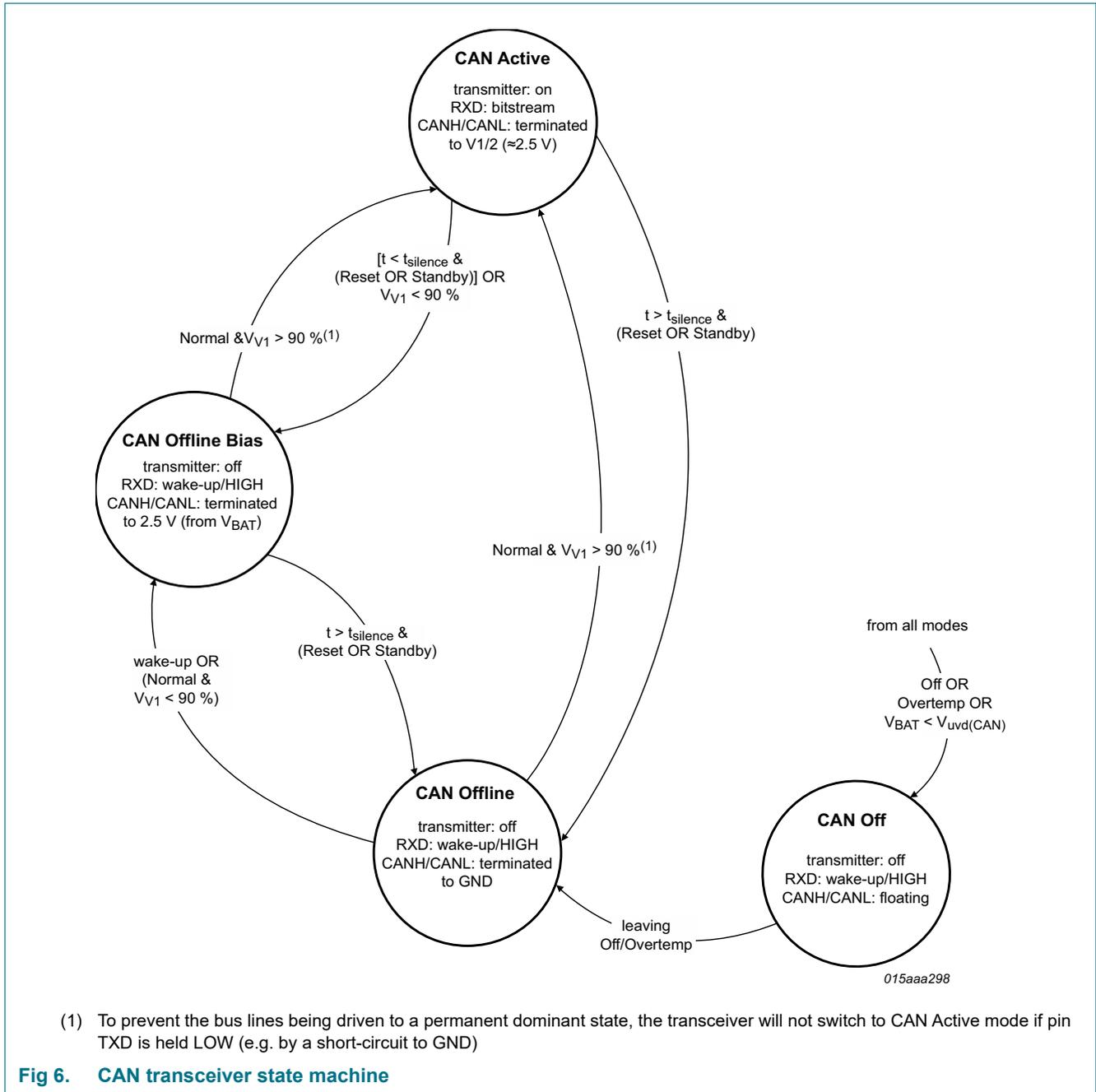
Fig 6. CAN transceiver state machine
