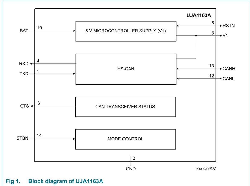
Fig 1. Block diagram of UJA1163A
