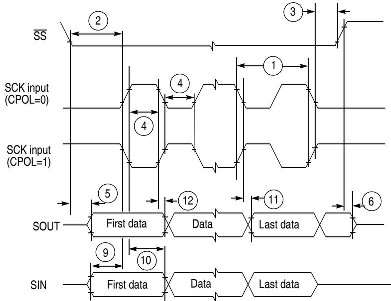
Figure 19. DSPI Classic SPI Timing—Slave, CPHA = 0
