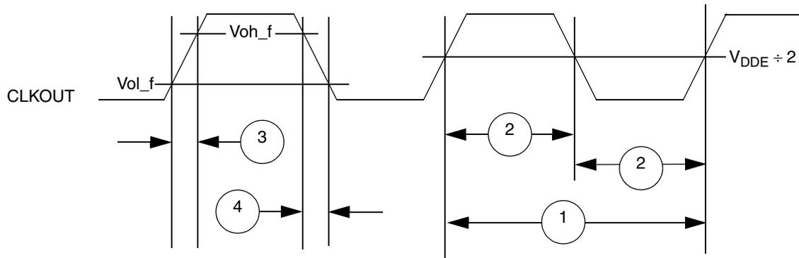
**Figure 12. CLKOUT Timing**
