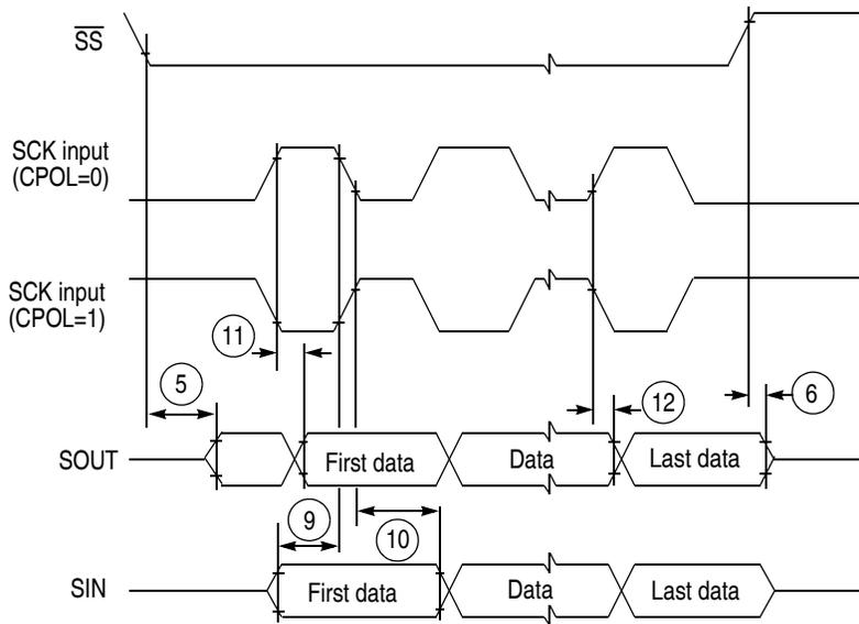
Figure 20. DSPI Classic SPI Timing—Slave, CPHA = 1
