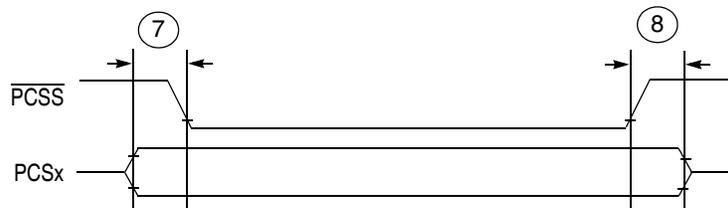
Figure 25. DSPI PCS Strobe ( $\overline{PCSS}$ ) Timing
