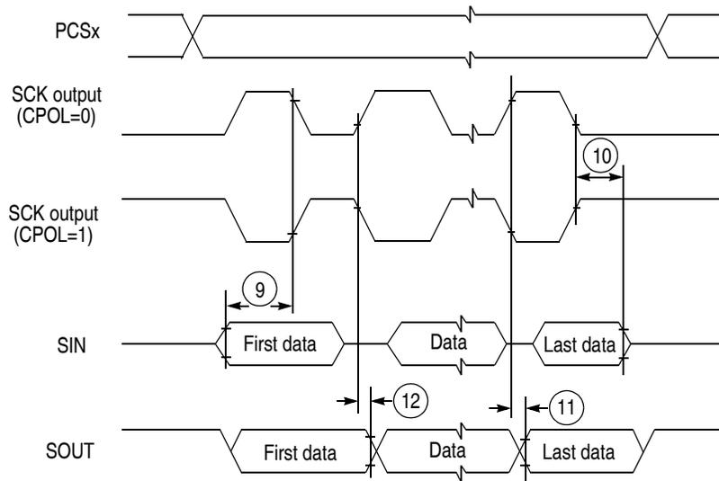
**Figure 18. DSPI Classic SPI Timing—Master, CPHA = 1**
