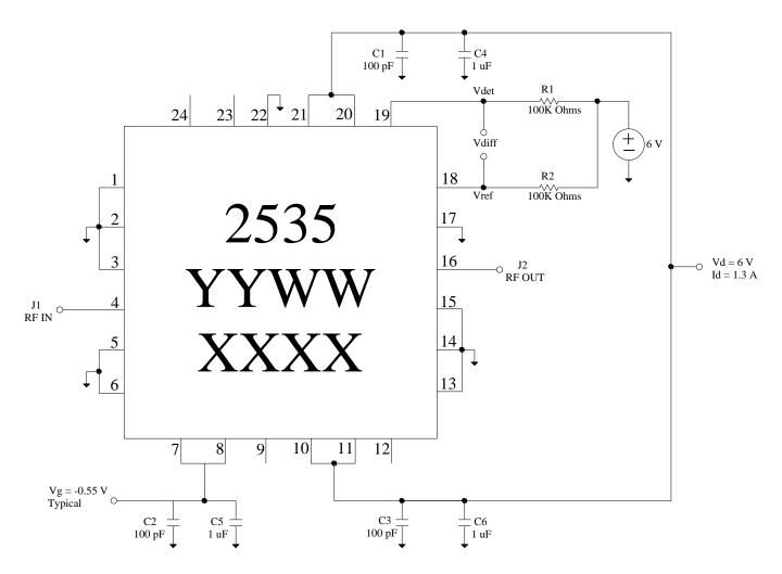
Vg can be biased from either side (pins 7 and 8 or pins 23 and 24), and the non-biased side can be left open. Vd must be biased from both sides (pins 10, 11, 20, and 21).
