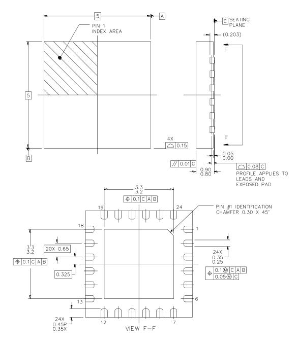
This package is lead-free/RoHS-compliant with a copper alloy base (CDA194), and the plating material on the leads is 100% matte Sn. It is compatible with both lead-free (maximum 260 °C reflow temperature) and tin-lead (maximum 245 °C reflow temperature) soldering processes.
