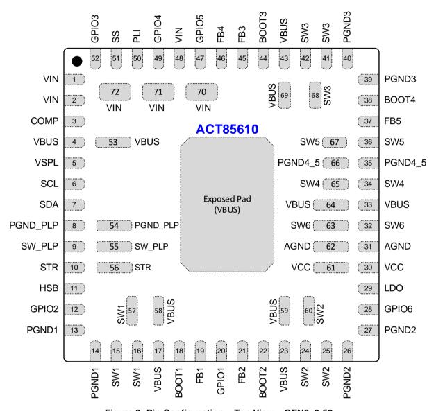
Figure 3: Pin Configuration – Top View – QFN6x6-52
