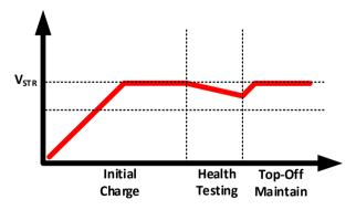
Figure 7: Storage Voltage at Different Stages
