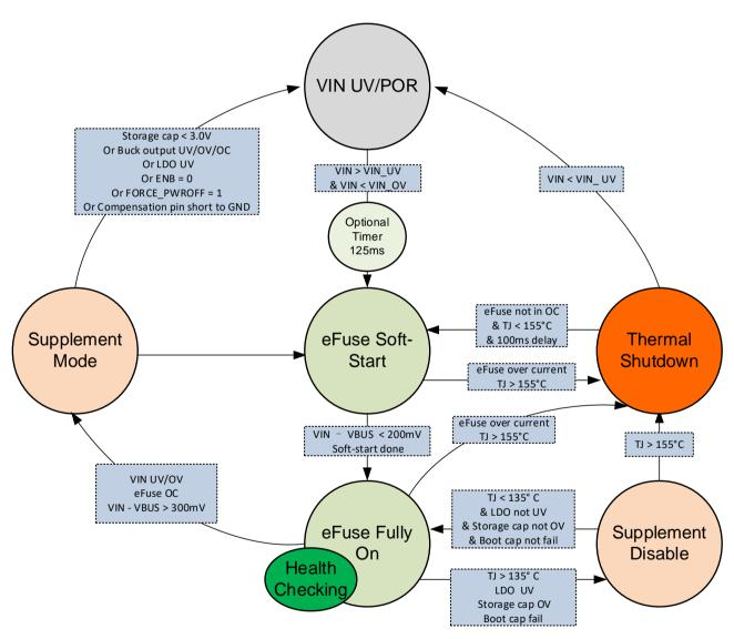
Figure 5: eFuse State Machine Diagram
