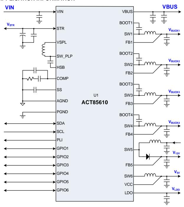
Figure 10: Application Schematic (12V Input)
