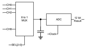
Figure 9: ADC Block Diagram
