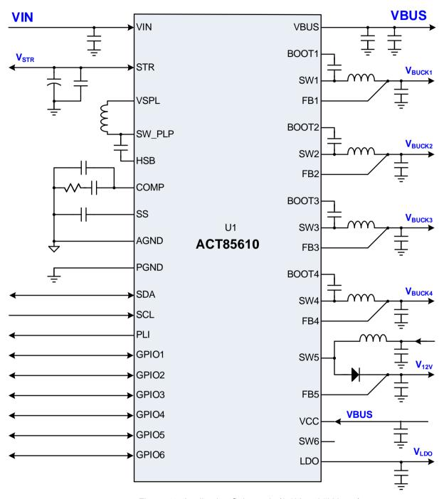
Figure 11: Application Schematic (3.3V and 5V Input)
