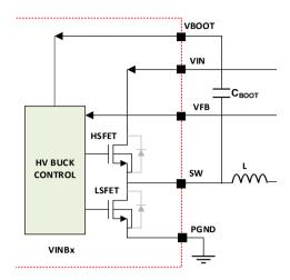
Figure 8: Buck Regulator Output Voltages
