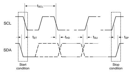
Figure 4: I<sup>2</sup>C Data Transfer
